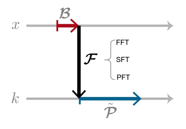
Many field solvers and functions are included in VirtualLab Fusion. They may either working in the space (x) domain or the spatial frequency (k) domain. To use different solvers and functions in connection, so to enable the modeling of complex systems, the transforming between x and k domain is a crucial step. Three Fourier transform algorithms are available in VirtualLab Fusion, and, with this document, we show how to set the options by discussing at different examples.
